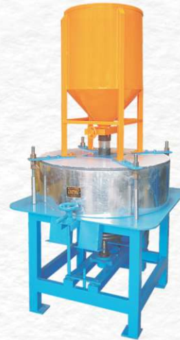
1200 MM - 48" MANUAL SHELLER FLOUR MILL
